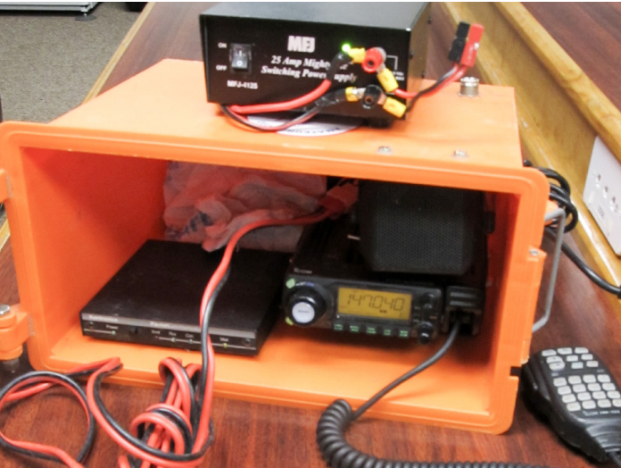
Above: PORTABLE AMATEUR RADIO— Polk County Coordinator Robert Herron shows how easy and inexpensive a licensed operator can construct an amateur radio and make it operative at any location. It can be used with a portable battery or regular current and is easily carried to different sites.
